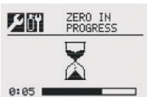
Figure 44. Zero Calibration in Progress
