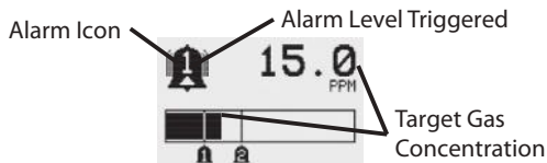
Figure 34. General Status Alarm - detail
