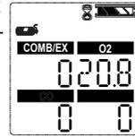
After the Bump Test completes, the device momentarily displays "BUMP PASS" or "BUMP ERROR" along with the label of any sensor that failed before returning to Measure mode. If the device fails the Bump Test, perform a calibration as described in chapter 3.9.
