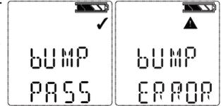
The ✓ symbol will be displayed in the Measure mode for 24 hours after a successful Bump Test.
