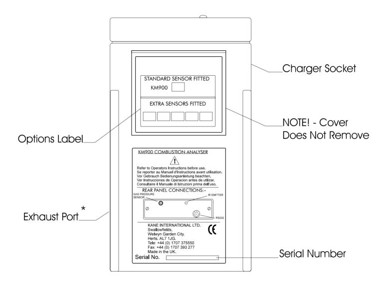
\*NOTE! Do not cover exhaust port as this will severely affect analyser operation
