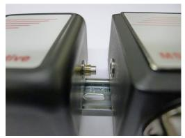
Replacement plated metal connector design linking the Satellite XT (right) to the Extractive module (left).
