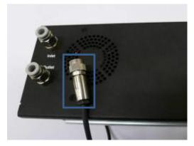
Revised Pyrolyzer module flying lead with fitted metal plug
