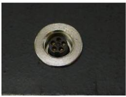
Detail of the revised Satellite XT plated metal socket for connection to the Extractive module
