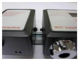
Previous black plastic connector design linking the Satellite XT (right) to the Extractive module (left).
