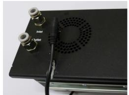
Previous Pyrolyzer module flying lead with moulded plug (black colour)
