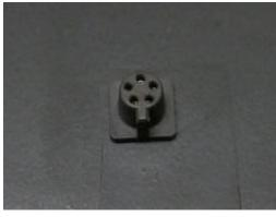
Detail of the previous Satellite XT black plastic connector for connection to the Extractive module
