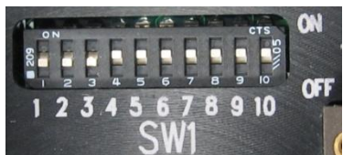
Figure 3-1 (SW1) Ten (10) Position DIP Switch
