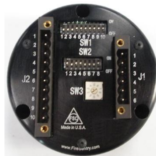
Figure 2-9 Detector Module “puck” (rear view)
