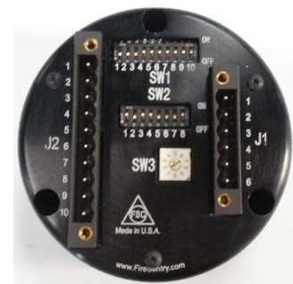
Figure 1-2 FS19X/FS20X Detector Puck, (rear view)
