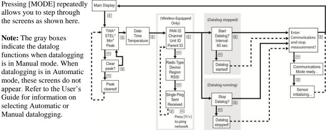
\* If your ToxiRAE Pro is configured with an oxygen (O2) sensor, TWA and STEL are not included in the menus because neither TWA nor STEL are calculated for this sensor. Min (for minimum) is included only when an oxygen sensor is used.
