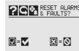
Figure 21. Alarm/Fault Reset Confirmation Screen
