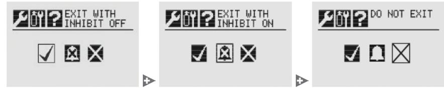
Figure 11. Exiting Zero Gas and Span Gas calibrations
