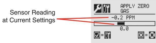
Figure 4. Zero Gas Calibration Screen
