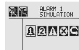
Figure 16. Alarm/Fault Simulation Menu
