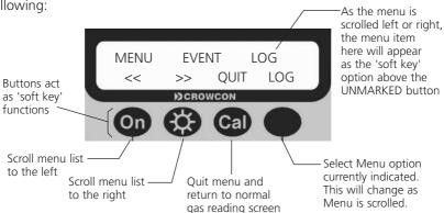
The four buttons have above them a symbol or word: these are the 'soft key' functions currently assigned to that particular key. Use the ON and BACKLIGHT buttons to scroll left and right, the CAL button to quit the menu system and the UNMARKED button to select a menu option. View the road map on page 37 for details of Detective+ IR configuration menu system
