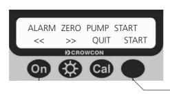
Press the UNMARKED button to enter the START submenu
