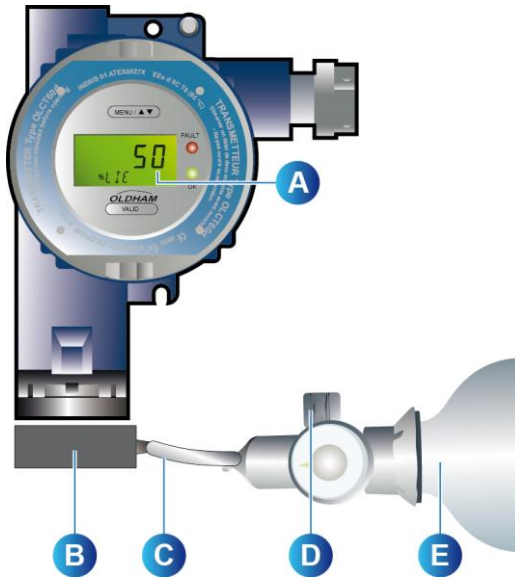
Figure 27: Checking gas sensitivity
