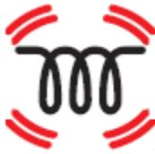
Heat Light: the adjacent light glows or flashes to indicate that power is being supplied to the elements
