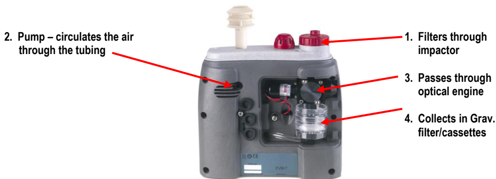
Figure 4-3: How the impactor functions
