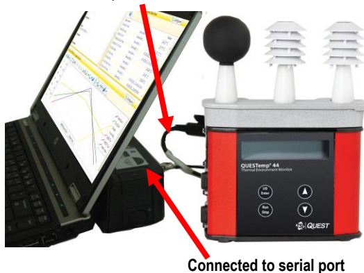
Figure 1-30: Communicating with the QT o 44/46 and DMS
