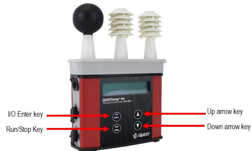
Figure 1-2: Keypad explained and identified
