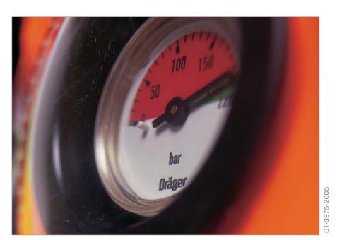
Check contents gauge ensuring the cylinder is fully pressurised (i.e. 200 bar). The gauge needle must be inside the green segment of the gauge face.
