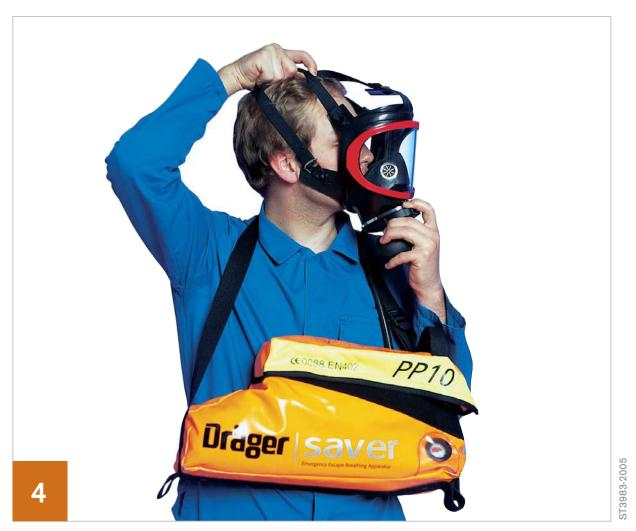
Donning the Face Piece. Using one hand, hold the facepiece onto the face and with the other hand, pull the elastic head harness over the back of head, locating the harness centrally with the back of the head.
