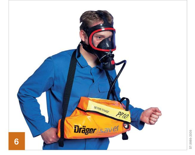
On achieving the face seal and on taking your first breath of inhalation the lung demand valve will automatically switch to positive pressure starting air supply to facepiece. Breathe normally and immediately leave the hazardous area by shortest and safest escape route.
