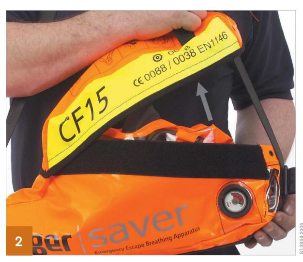
Grip the loop on the lid of the carrying bag and pull firmly upward to break the anti-tamper tag. Open the flap of the bag which then releases the locking clip from the valve turning on the air supply to the hood.
