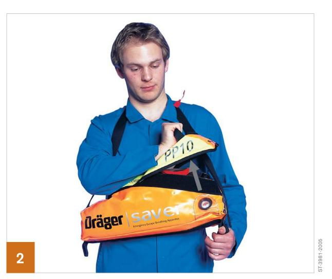
Grip the loop on the lid of the carrying bag and pull firmly upward to break the anti-tamper tag. Open the flap of the bag which then releases the locking clip from the valve turning on the air supply to the head.
