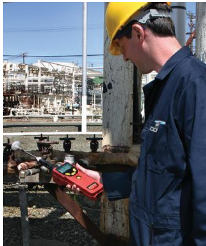
Workers can easily and quickly obtain VOC readings anywhere in the facility with the RAE Systems UltraRAE 3000+
