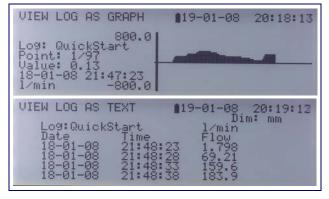
If logging is taking place at a 'named site' the log is saved with same 'name' as the site name and can be recalled under that name as and when required. This allows the instrument to be used at several site locations and the results can be downloaded independently at a later, convenient time.
