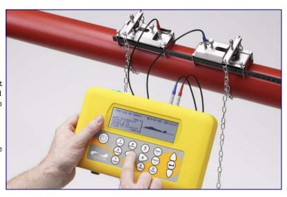
The PF330 is very much designed with 'ease of use' in mind. An interactive QuickStart menu, which simplifies system installation at any suitable location, together with minimal set-up requirements, means that the system can be installed and brought into service very quickly. Furthermore, the application parameters for a particular site can be saved to non-volatile memory and instantly recalled if a site is revisited for monitoring at a later time – further reducing the set-up time.
