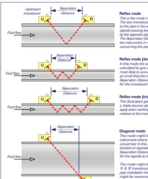
This is the mode most commonly used. The two transducers (U & D) are attached to the pipe in line with each other and the signals passing between them are reflected by the opposite pipe wall.
